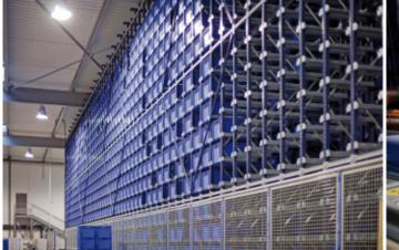
All processes related to picking begin in this area and are guided by the Mecalux Easy WMS warehouse management system. The first step is placing the boxes in the order prep positions located at the back and that also form part of the conveyor.
