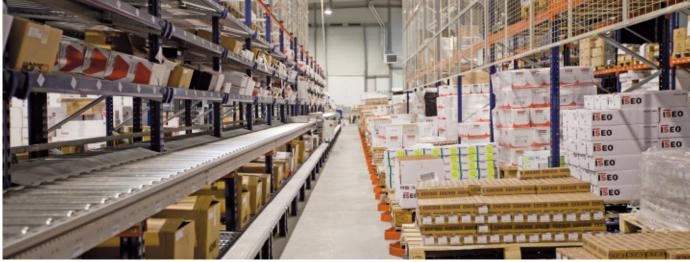
The automatic conveyor passes through the inside of the racks, between levels one and two. A second conveyor was installed, outside and in parallel to the racks, which is used as a prep table.
