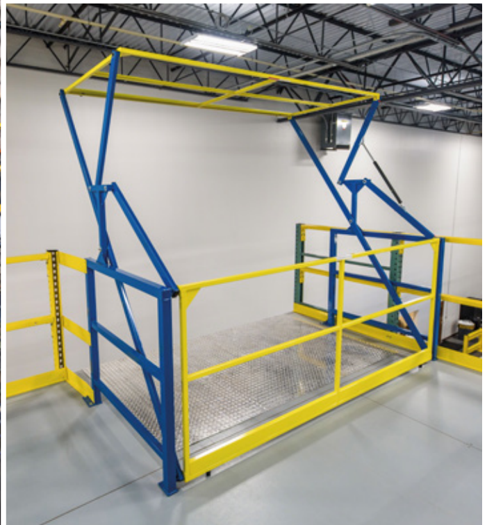
Additionally, up and over gates were enabled to create a loading and unloading zone for the goods handled by forklifts.
