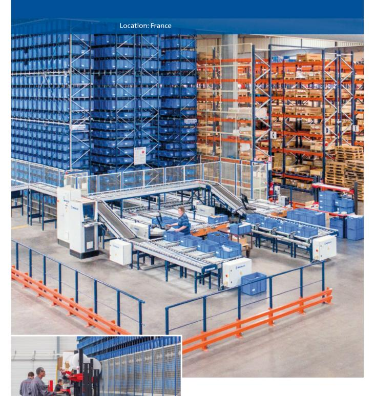
The new Grégoire-Besson logistics centre, a French farm technology equipment company, consists of an automated warehouse for boxes, pallet racking and cantilever racking by Mecalux. The combination of these three storage systems lets merchandise be organised according to their characteristics and demand, streamlining order picking tremendously.
