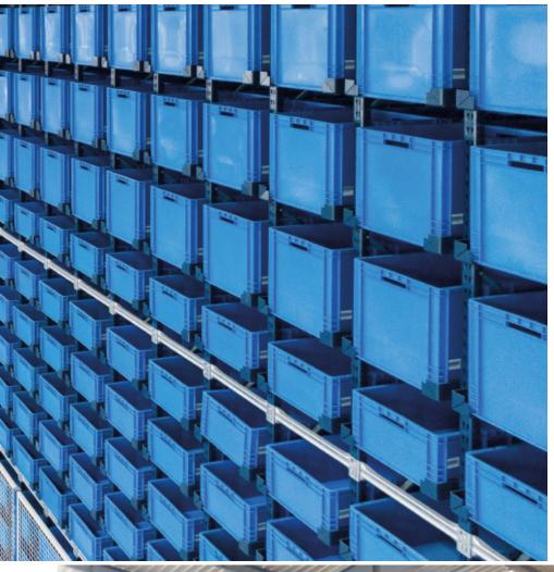
The racks have a storage capacity for 5,920 boxes of 600 x 400 x 240 mm and 4,144 boxes of 600 x 400 x 420 mm, which adds up to a total of 10,064 boxes of small-sized items
