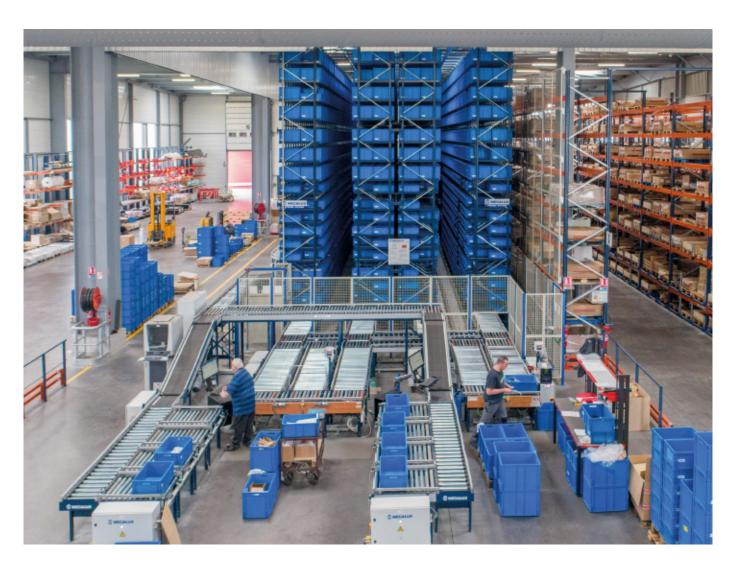
The warehouse is composed of two aisles with double-deep racking on both sides that measure 47 m long, 9 m high and have 17 shelves.
