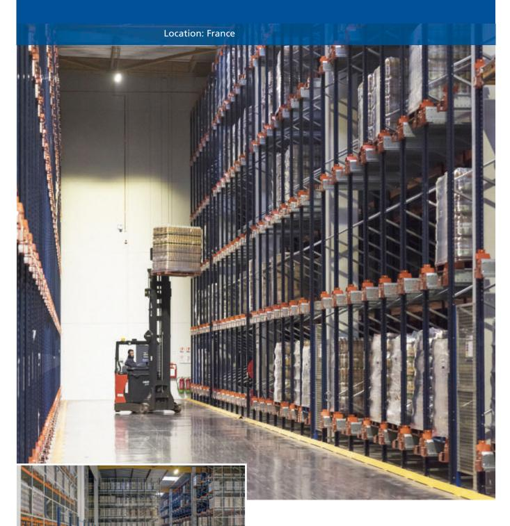
Grupo Alainé has expanded its Mâcon installations (in France) to accommodate the new production line of one of its customers. To do so, Mecalux has equipped an 8,000 m² floor area with the semi-automatic Pallet Shuttle system that offers a total 20,397-pallet storage capacity. This solution is ideal for housing large volumes of pallets per SKU in channels that run up to 43 m in depth, as well as for managing the loading and unloading of 2,500 pallets a day.
