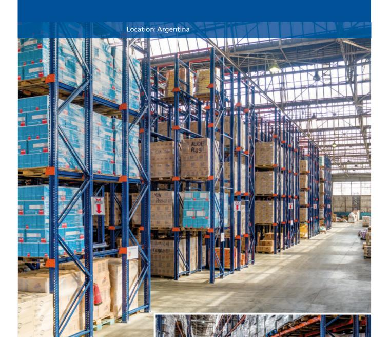
The wholesale company Caromar has inaugurated a distribution centre in La Tablada (Buenos Aires) with the intent to increase storage capacity and, simultaneously, provide quality service at the lowest possible cost. Mecalux has equipped it with pallet racks and drive-in racks, which provide capacity for 9,728 pallets.
