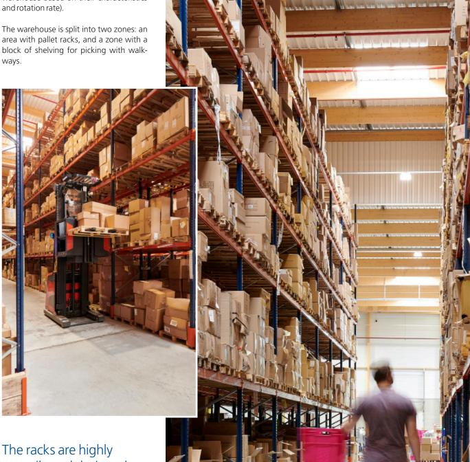
versatile and designed to store pallets of different sizes, weights and shapes
