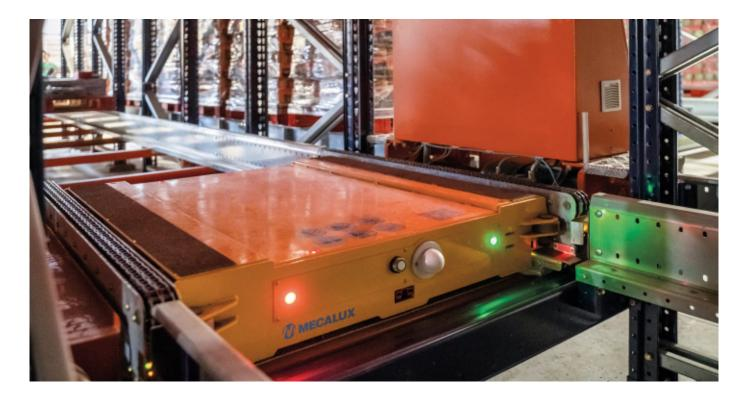
Two transfer cars organise the pallets and sort them into 19 live preload channels depending on the order or route. The pallets remain in these channels, waiting for the operators to load them into the lorries.
