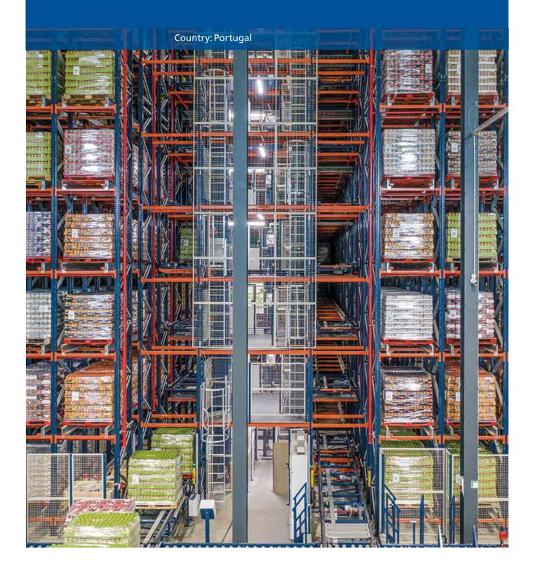
Cistér, a Portuguese producer of pulses, has decided to automate its logistics processes to modernise and improve its supply chain. With the collaboration of Mecalux, the firm has set up the automatic Pallet Shuttle system with transfer cars in its new warehouse in Alcobaça (Portugal). The storage capacity is 12,672 pallets. The warehouse, connected to the production plant via a conveyor circuit, is managed by Easy WMS.
