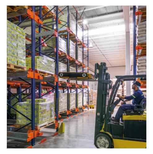
In view of this request, Mecalux proposed equipping the warehouse with high-density racks with the semi-automatic Pallet Shuttle system for two reasons: for one thing, the racks take advantage of the available warehouse space and provide as much storage capacity as possible and, for another, this solution greatly streamlines storage tasks.
