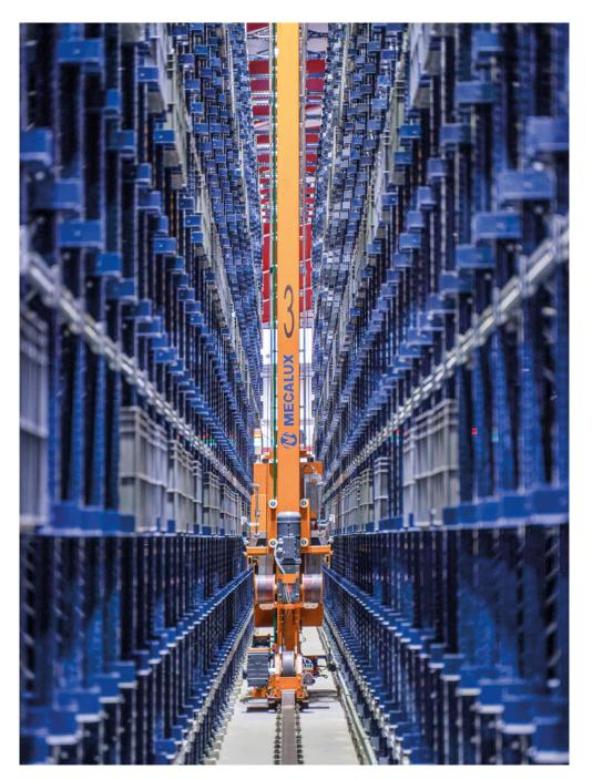
The miniload stacker crane moves boxes at a travel speed of 250 m/min
