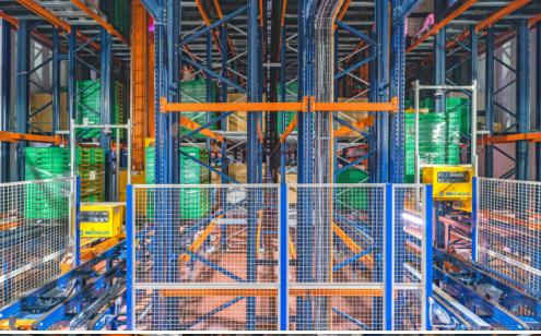
The automated storage and retrieval systems ensure proper product handling and facilitate the work of the operators
