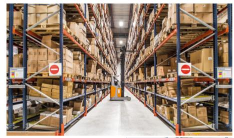
Operators criss-cross the aisles with the hand-held terminal and the warehouse management software indicates which items must be collected.
