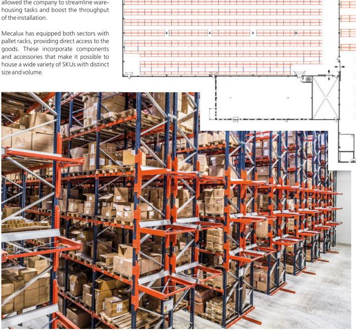
One of the sectors has narrow aisles. Consequently, these operate by turret trucks. When carrying out picking, high-reaching order pickers are used.
