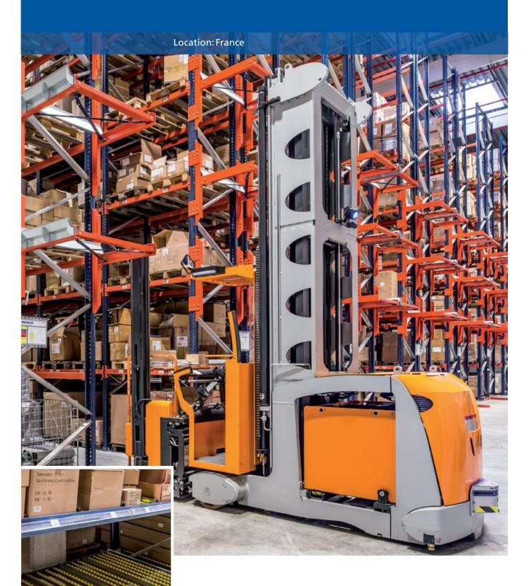
The 8,900 m<sup>2</sup> logistics centre of the French company Côté Table is sectored into two different areas. Mecalux has installed pallet racking in both zones, with a storage capacity of more than 19,600 pallets. Designed specifically for the picking of orders, the warehouse increases the speed of this primary operation.
