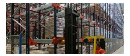
Workers deposit the Pallet Shuttle in the corresponding channel. Soon afterward, they insert the goods in the channel's first position and the motorised shuttle takes it directly up to the first open location it finds inside the channel. Operators use a tablet with a WiFi connection to interact with the shuttles and organise the introduction and extraction of the pallets. And, seeing that operators do not need to enter the lanes to handle the goods, this reduces potential damage to the racks.
