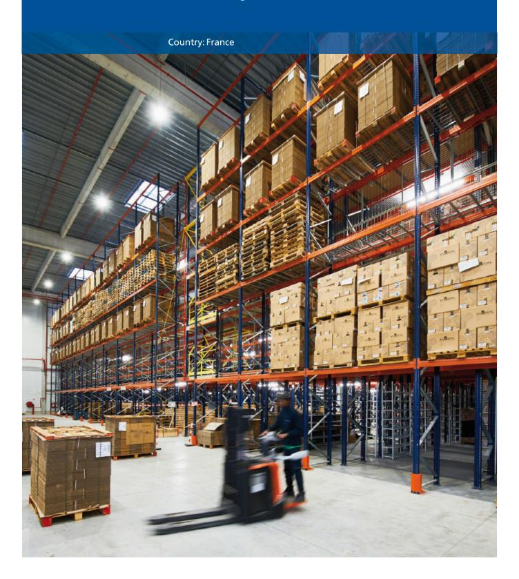
Mecalux has equipped one of the Everial document centre's warehouses in Lyon (France) with racks with walkways. Overall, they provide capacity for 360,000 boxes and consist of five floors. This storage system is notable for making full use of the entire surface area and for its simplicity, while also making file searching and handling much faster.
