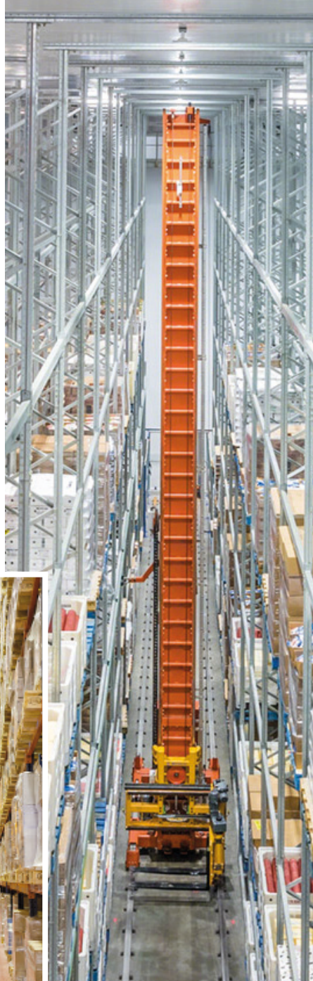
Automatic trilateral stacker crane
