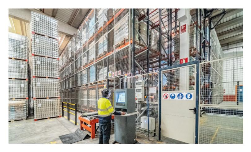
er crane. This high-density automated storage and retrieval system (AS/RS) has boosted efficiency in the Envases Group facility. In addition to making the most of its floor space to expand storage capacity, the company has leveraged automation to streamline and maintain stricter control over incoming and outgoing goods.
