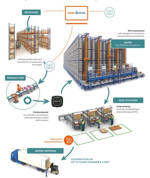
Based on this message, Easy WMS uses a set of rules and algorithms to assign a location to each item according to its attributes and turnover rate.
